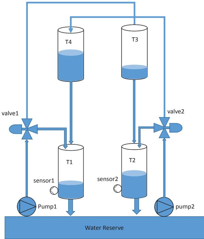
Figure 2 Diagrammatic representation of the four-tank process
