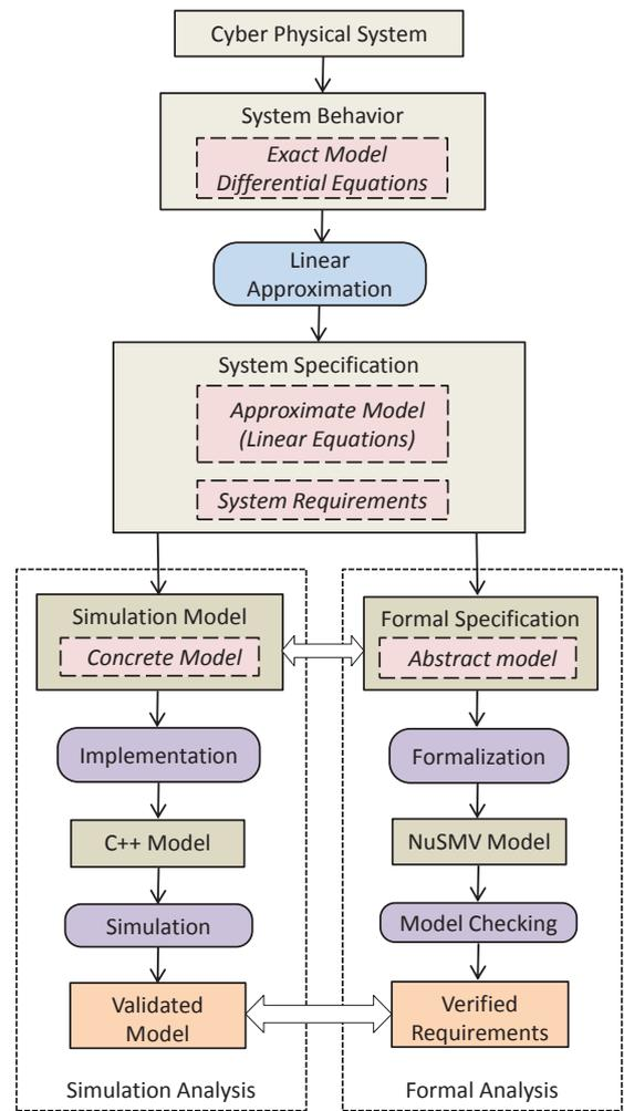
Figure 1 Proposed CPS System Analysis Methodology
